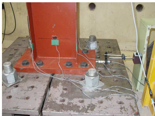
Fig. 3. Column base connection and strain gauge.
