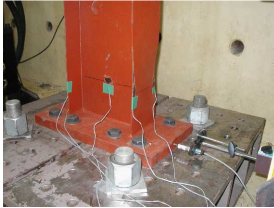
Fig. 10. Local buckling of the column ② at the base level (test frame no. 2).
