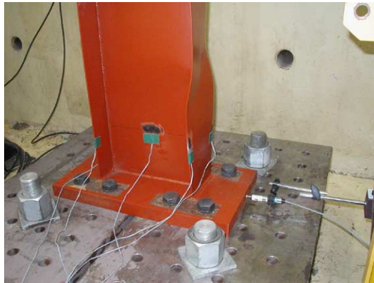
Fig. 11. Local buckling of the column ② at the base level (test frame no. 3).
