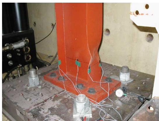
Fig. 9. Local buckling of the column ② at the base level (test frame no. 1).
